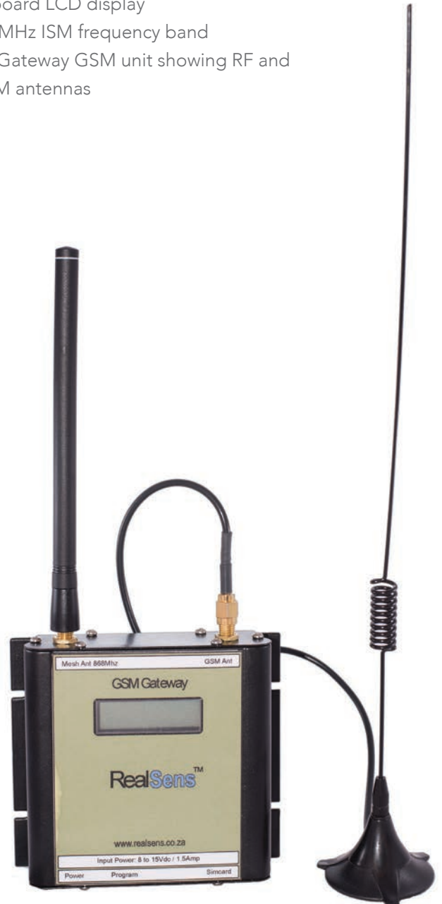
RS-Gateway GSM unit showing RF and GSM antennas
