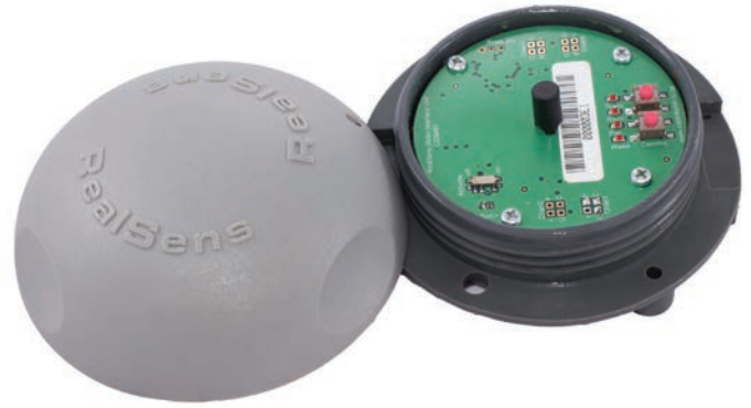
RS-MIU with top screwed on (left) and off (right), showing PC board with RF antenna and diagnostics buttons
