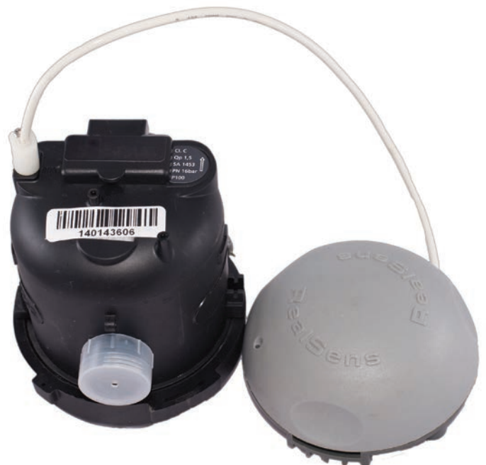
MIU connected to meter
